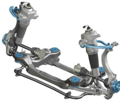
**Fig. 16. Front suspension**
