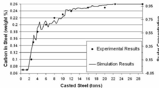
Fig. 5: Carbon content during a steel change situation in tundish with flow control device.
